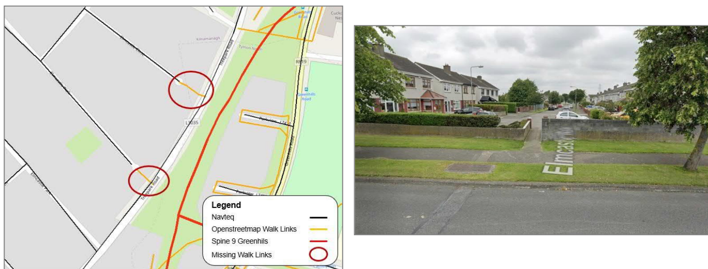
Figure 4.2 Example of permeability link missing from Navteq mapping on Tallaght/Clondalkin Cor Bus Corridor.
